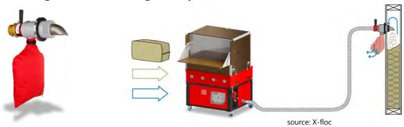
In the case of small or air-impermeable constructions (e.g. under windows and jambs, interior walls, etc.), it is recommended to use a venting rotary nozzle.
