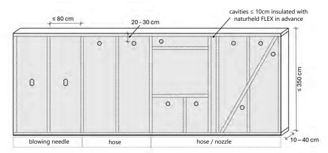
Defined holes of 105 or 120 mm are only required when using sealing plugs.
