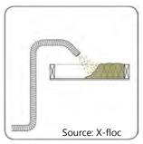
With open inflation, the thermal insulation material is applied to a surface that is open at the top. The top storey ceiling or vaulted ceilings are often insulated in this way. In the simplest case, it can be applied using a hose or a rigid pipe.
