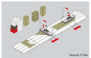
With partially and fully automated stationary filling technology, wall, ceiling and roof elements planked on one side are filled on transport tables with a blow -in panel from the upper, still open side.
