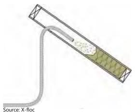
Filling with an injection hose is probably the best-known method. A distinction is made between transport and delivery hoses and the injection hose.
